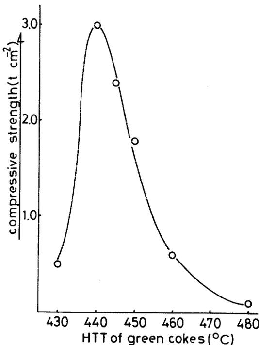
Figure 8 Compressive strength of the moulded discs calcined at 1200°C.
