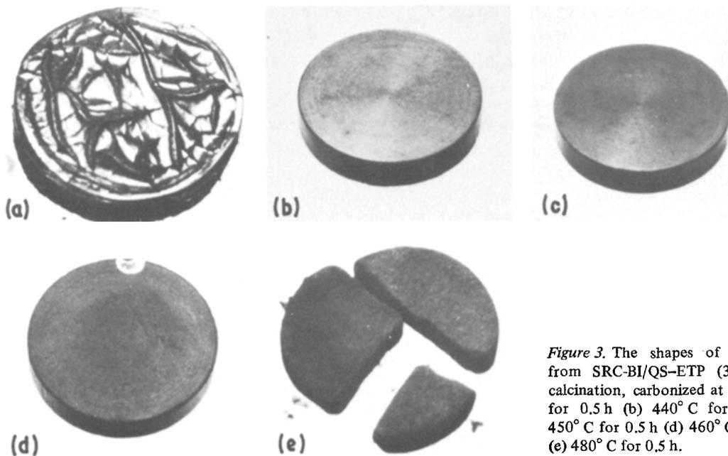
**Figure 3.** The shapes of the disks from SRC-BI/QS-ETP (3-2), after calcination, carbonized at (a)  $430^\circ \text{ C}$  for 0.5 h (b)  $440^\circ \text{ C}$  for 0.5 h (c)  $450^\circ \text{ C}$  for 0.5 h (d)  $460^\circ \text{ C}$  for 0.5 h (e)  $480^\circ \text{ C}$  for 0.5 h.
