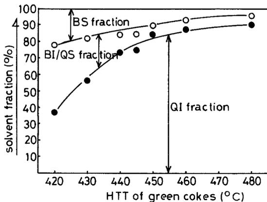
Figure 6 Relationship between carbonization temperature and solvent fractionation yield of green cokes prepared at variable temperatures.
