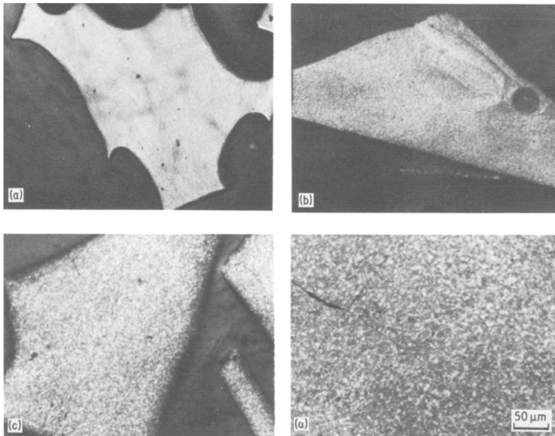
*Figure 1* Optical micrographs, using crossed-Nicols, of cokes obtained from single carbonization and co-carbonization with SRC-BI/QS and ETP. ( $150^{\circ}\text{C h}^{-1}$  heating rate, carbonized at  $600^{\circ}\text{C}$  for 2 h) (a) SRC-BI/QS washed with a THF-Benzene mixture (mixing ratio = 1-4), (b) SRC-BI/QS, (c) SRC-BI/QS-ETP (3-2), (d) SRC-BI/QS-ETP (2-3).
