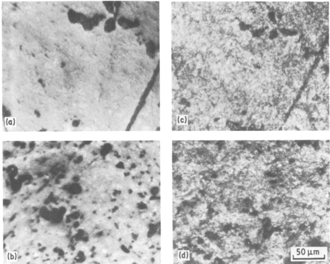
**Figure 2** Optical micrographs using crossed-Nicols, of the surface of discs moulded under  $400 \text{ kg cm}^{-2}$  from SRC-BI/QS and ETP (3-2) (a) before calcining, carbonized at  $440^\circ \text{ C}$  for 0.5 h, (b) before calcining, carbonized at  $450^\circ \text{ C}$  for 0.5 h, (c) after calcining, carbonized at  $440^\circ \text{ C}$  for 0.5 h, (d) after calcining, carbonized at  $450^\circ \text{ C}$  for 0.5 h.
