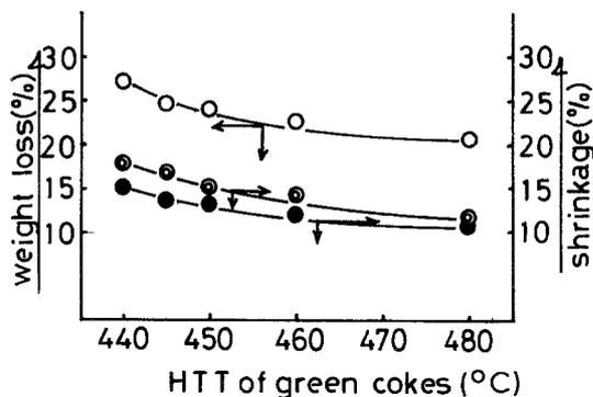
Figure 7 Relationship between weight loss and shrinkage ratio of the discs by calcination at 1200°C ○: weight-loss, ○: diameter shrinkage, ●: thickness shrinkage.
